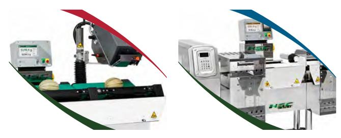
Standard "**peak weight**" checkweighers need a gap between products being a little longer than the weighing conveyor. **EasyWeigh**<sup>®</sup> checkweighers, on the contrary, just need the pitch between two products to be a little greater than the weighing conveyor's length.
