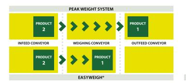
**EasyWeigh**<sup>®</sup> technology allows to weigh every new product regardless from the shape, format or line orientation without the need for any calibration or learning procedures.
