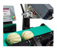
**Round Products Labeler** Special top labeler's architecture with pairs of **reclinable twin belts**, for the ideal application.
