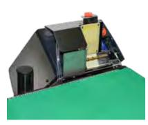
Side Labeler The label is placed on the lateral face of the products, applied by an air compressed blast.
