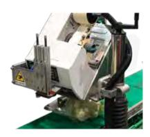
Pneumatic Arm Labeler The label is placed on the top face of the products, applied by a pneumatic labeling arm.
