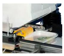
**"C" Labeler** The label wraps the product from the top face to the bottom, while running **through the applicator.**
