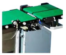
Bottom Labeler The label is placed on the bottom face of the products, running over the applicator.
